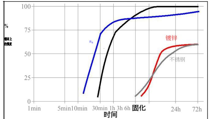
**固化速度与粘接间隙的关系**
